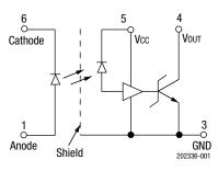
Figure 1. OLI500 Block Diagram
