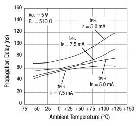
Figure 5. Propagation Delay vs Temperature
