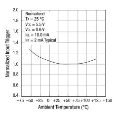
Figure 3. Normalized Input Trigger Current vs Temperature
